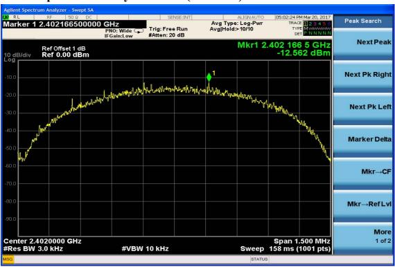
**Power Spectral Density Test Plot (CH-Mid)**
