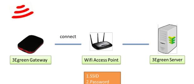
Gateway need connect with Wifi AP, then data can pass on sent to cloud servor. Gateway need know Wifi AP SSID and Password, the Gateway APP function is to set the parameter into Gateway  $^{\circ}$
