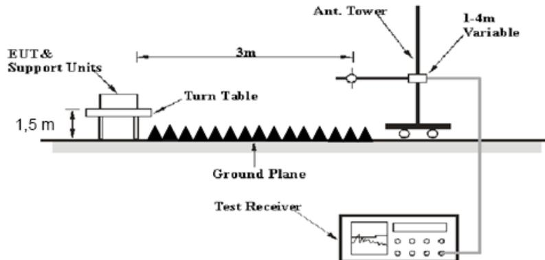
The radiated emission tests were performed in the 10 meters chamber test site for the range 30MHz to 1GHz and the 3 meters chamber B test site for above 1GHz, using the setup accordance with the ANSI C63.10-2013. The specification used was the FCC 15.209, and FCC 15.247 limits.
