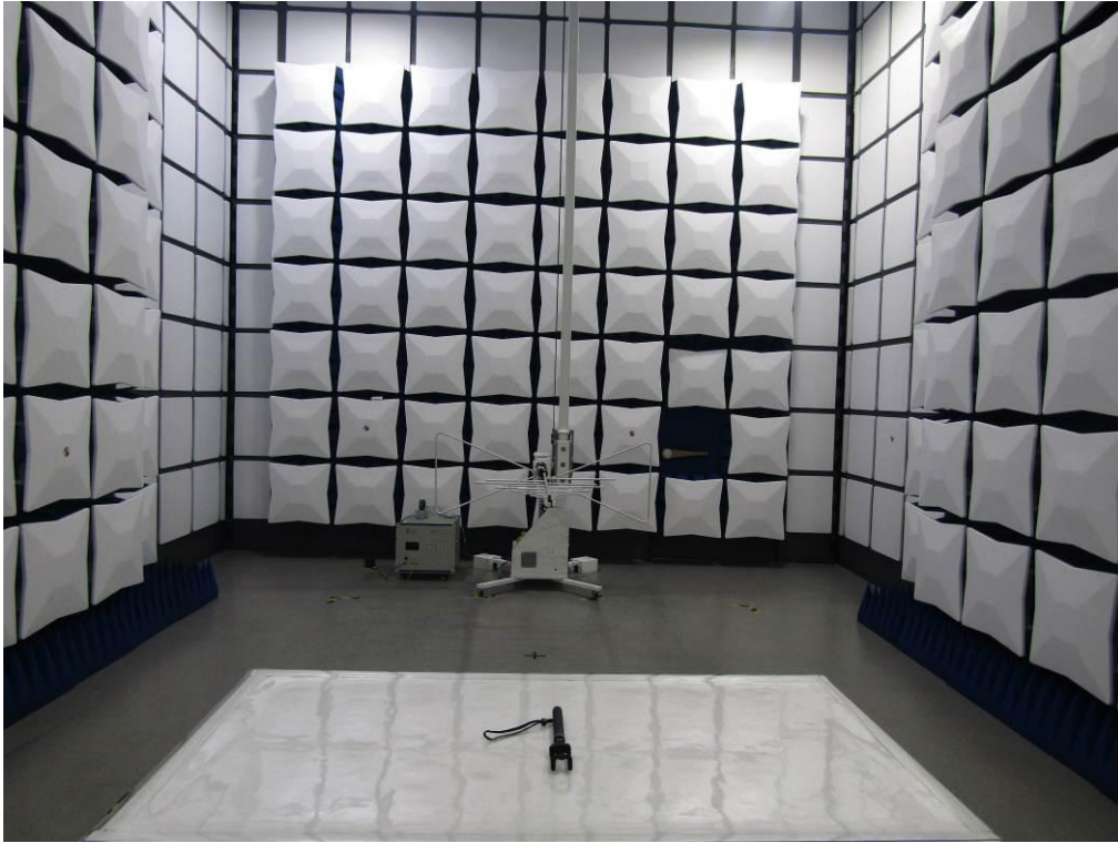
FCC RADIATED EMISSION TEST SETUP
