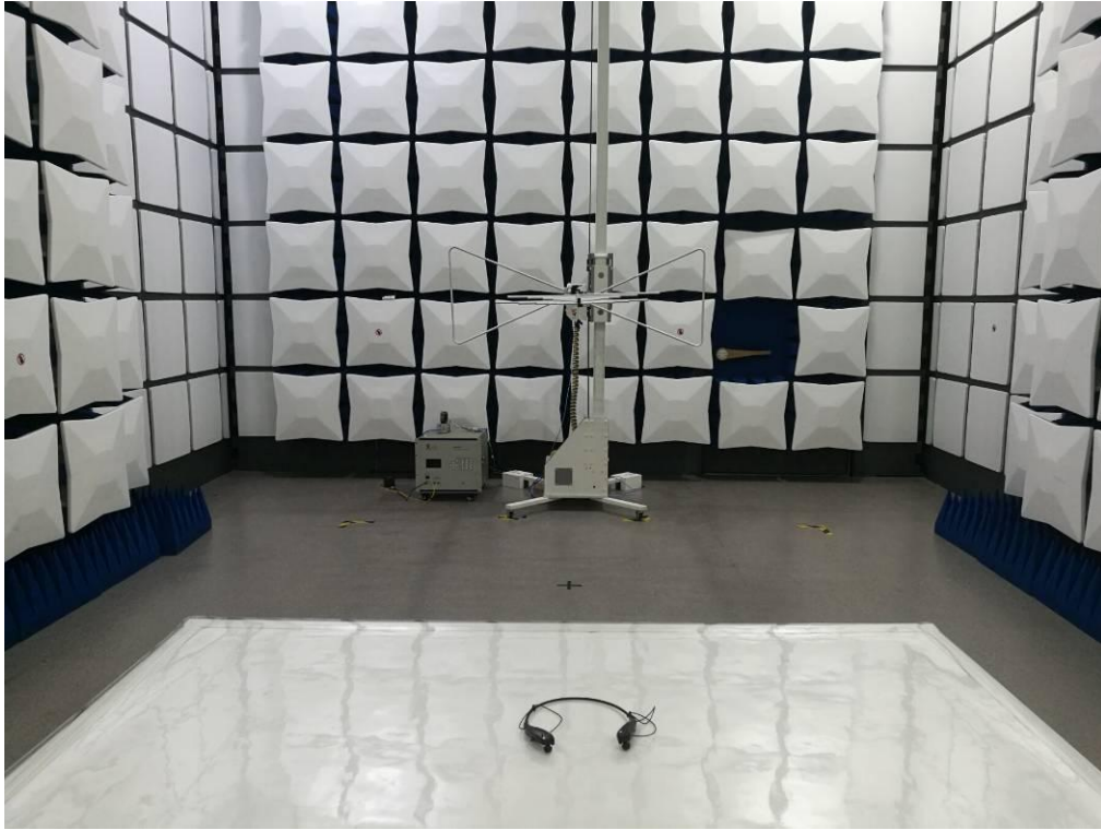
FCC RADIATED EMISSION TEST SETUP
