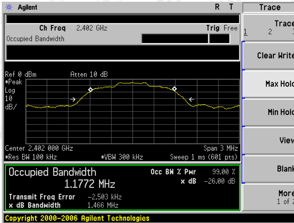
TEST PLOT OF BANDWIDTH FOR LOW CHANNEL
