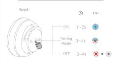
Long press it for 4 seconds to enter the pairing mode. Meanwhile, the red and blue indicator lights flash alternately. Turn on the Blue tooth of the mobile phone, search the Bluetooth device and find "Mpow H1" in the list to connect it. When it doesn't connect to the Bluetooth device of the phone, it will power off automatically after 10 minutes. Voice Dial Continuously double press it to enter voice dial.
