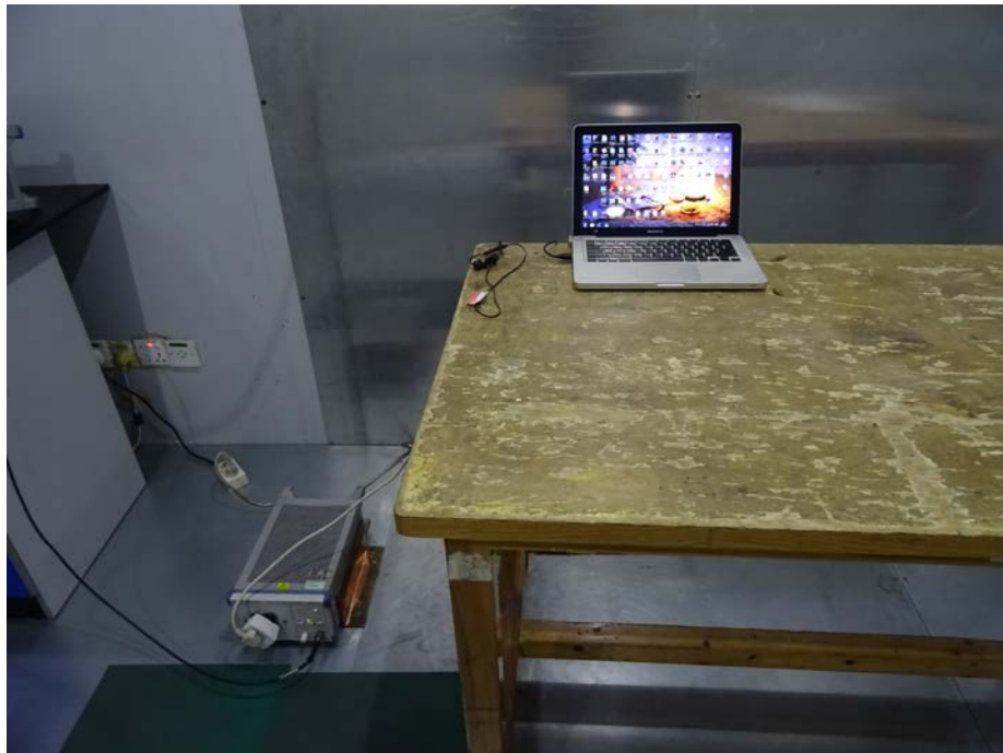
Photograph – Conducted Emission Test Setup
