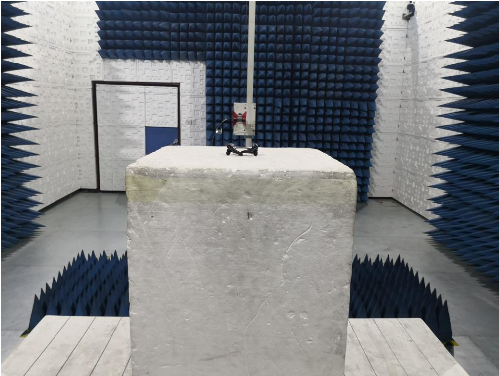
RADIATED EMISSION TEST SETUP ABOVE 1GHZ
