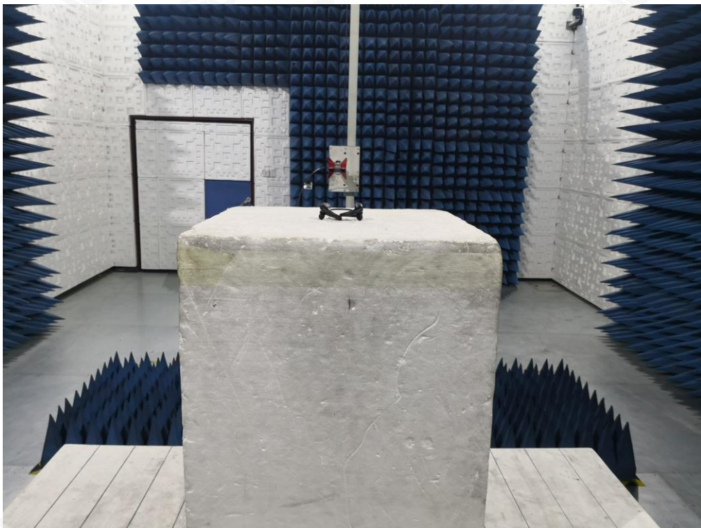
RADIATED EMISSION TEST SETUP ABOVE 1GHZ
