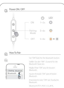
Shutdown state , Long press Power button for "3~45" ,enter pairing mode directly.
