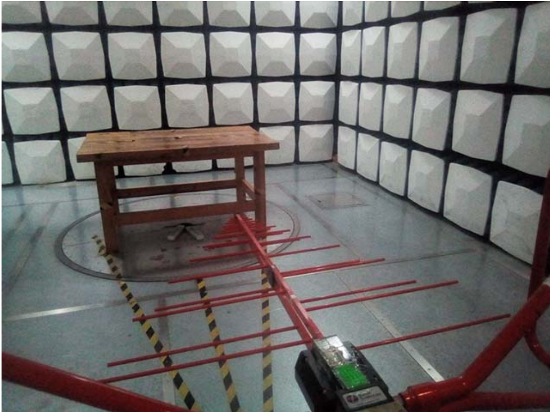
Radiated Emission Above 1GHz View
