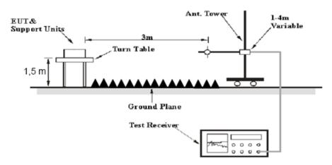
The radiated emission below 1GHz tests were performed in the 10 meters chamber test site, above 1GHz tests were performed in the 3 meters chamber test site A, using the setup accordance with the ANSI C63.10-2013. The specification used was the FCC 15.209, and FCC 15.247 and the RSS-247 Clause 5.5, RSS-GEN Clause 8.10 limits.
