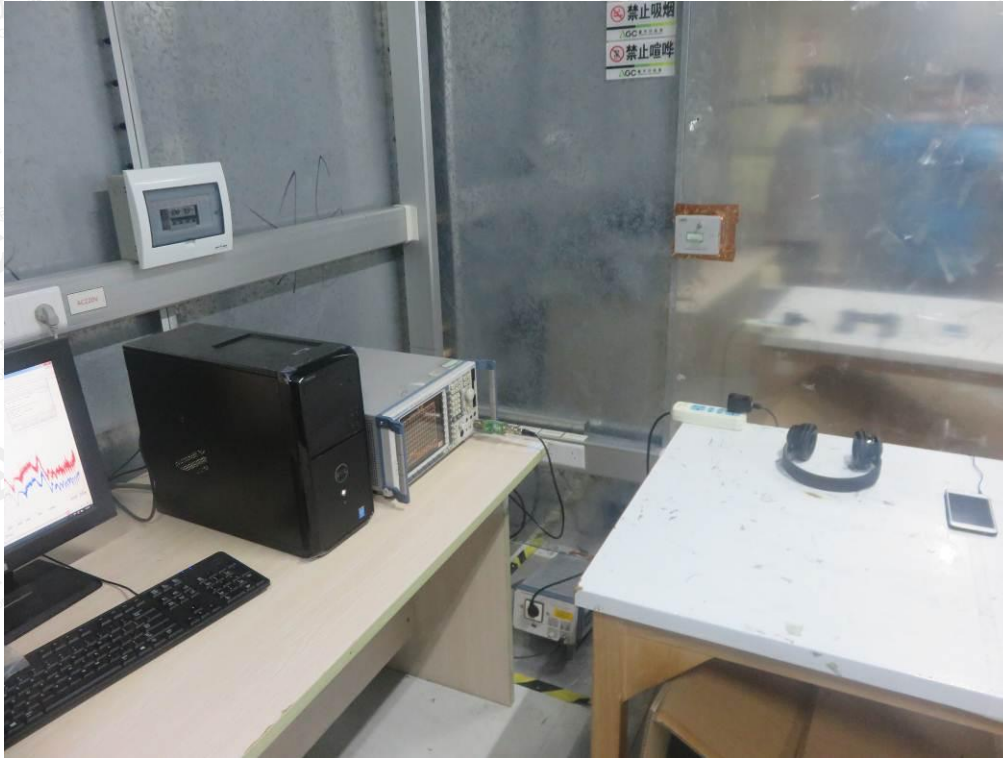
FCC RADIATED EMISSION TEST SETUP
