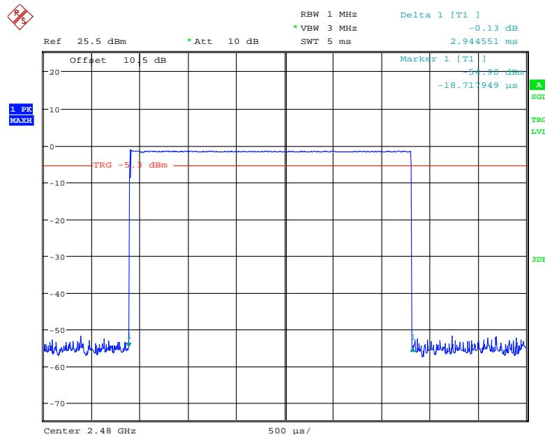
**EDR ( $\pi/4$ -DQPSK):****Pulse time, Low Channel, 2DH1**
