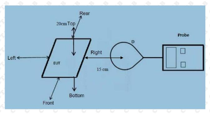
Note: Measurements should be made from all sides and the top of the primary/client pair, with the 15 cm measured from the center of the probe(s) to the edge of the device
