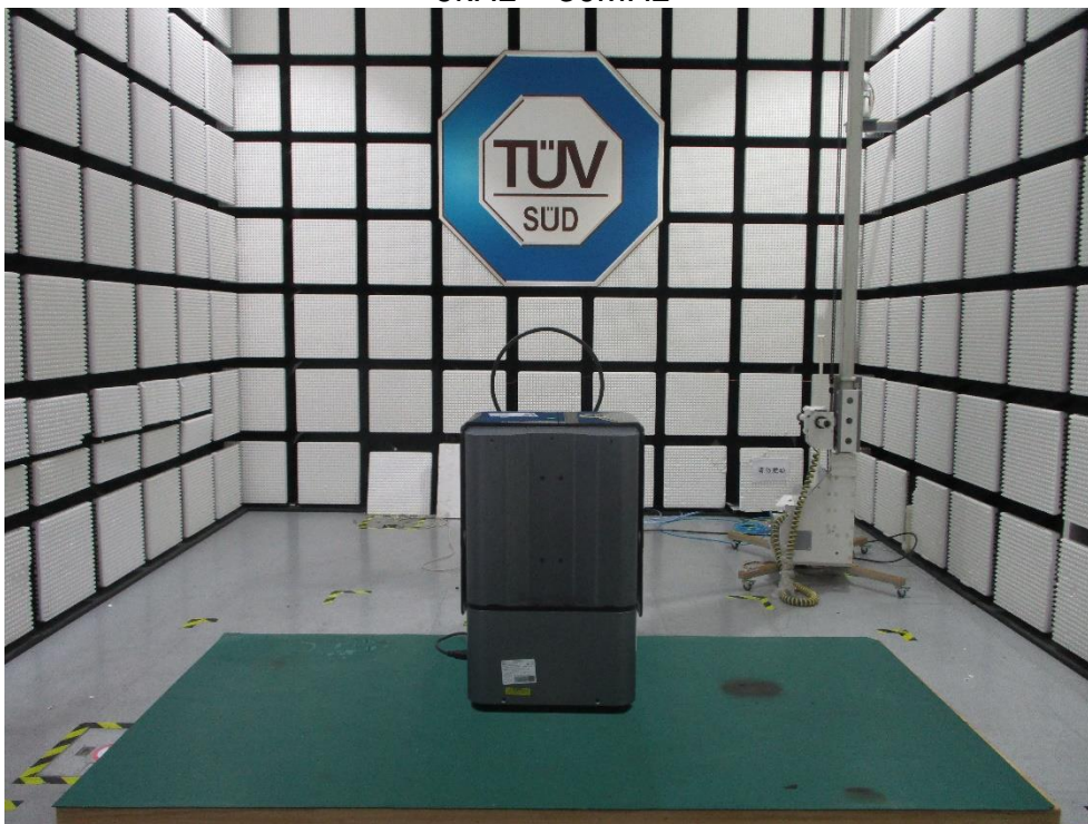
Radiated Emission Setup 9kHz ~ 30MHz
