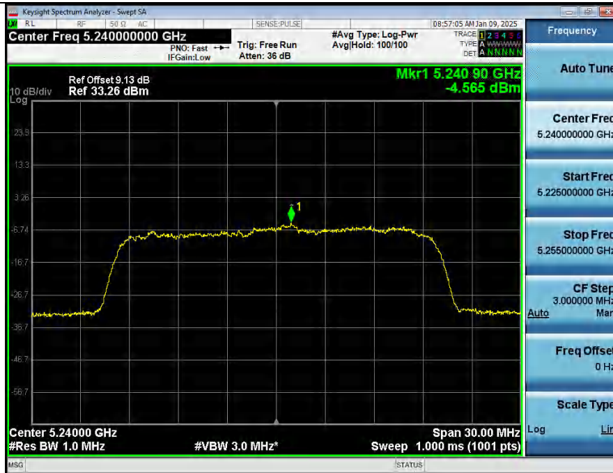
Power Spectral Density NVNT_ANT2_802_11n(HT20)_5240
