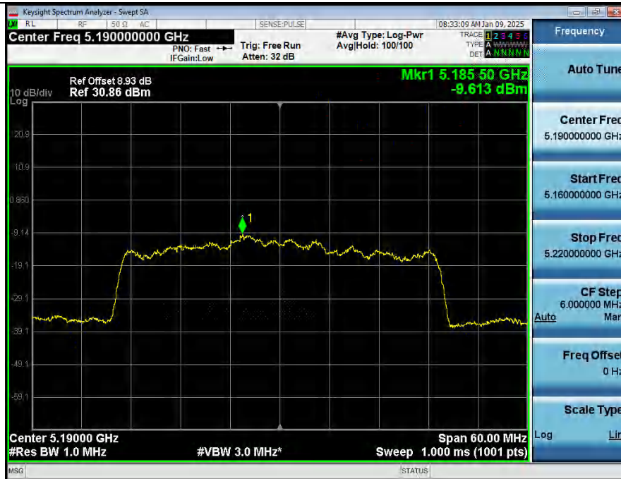
Power Spectral Density NVNT_ANT2_802_11n(HT40)_5190
