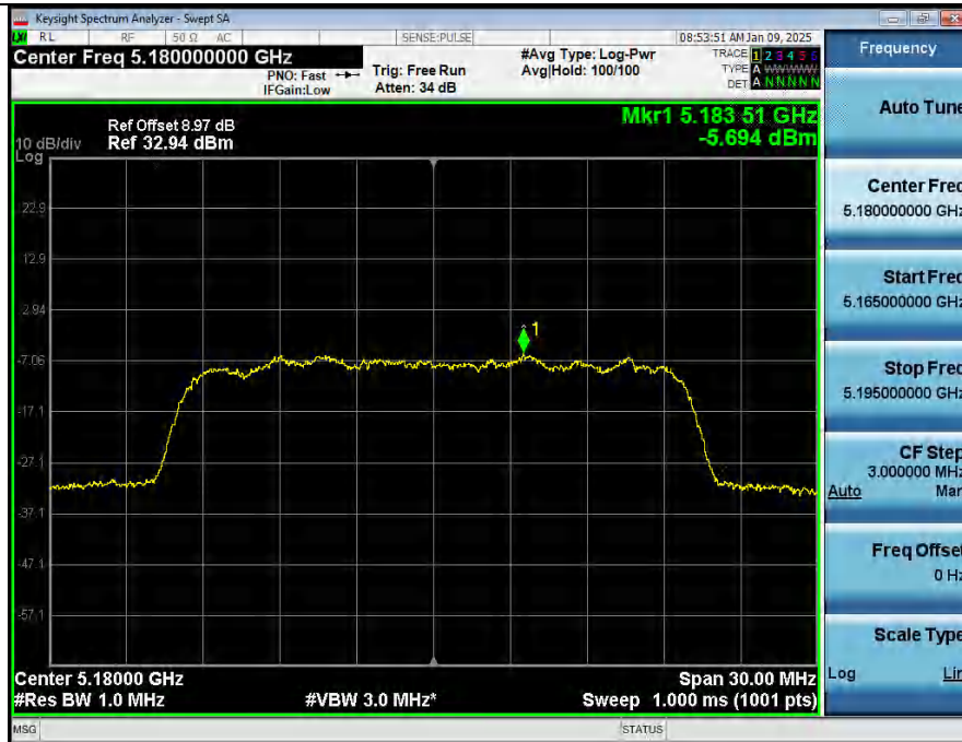
Power Spectral Density NVNT_ANT2_802_11n(HT20)_5180
