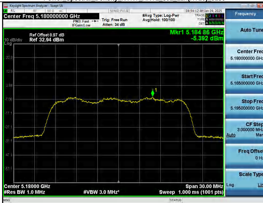
Power Spectral Density NVNT_ANT2_802_11n(HT20)_5180
