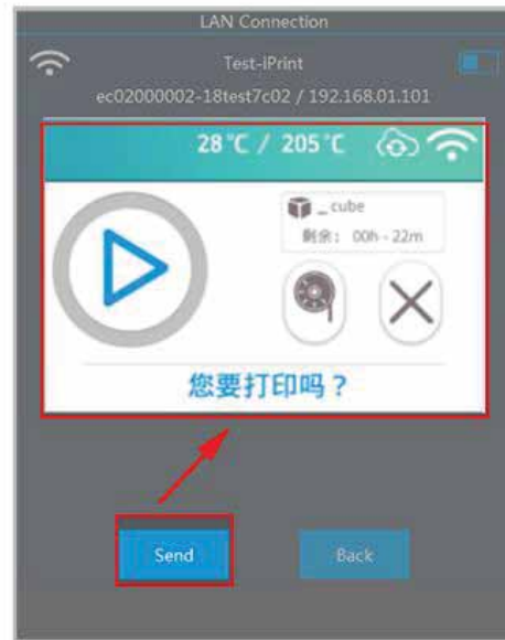
Step4:Use "Send file " to send local .gsd file to printer via LAN to print. You can monitor the whole printing process on PC software.
