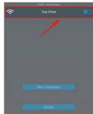
Step3:Use " LAN link " function in 3dstar and make sure the WIFI name is the same one PC connected.
