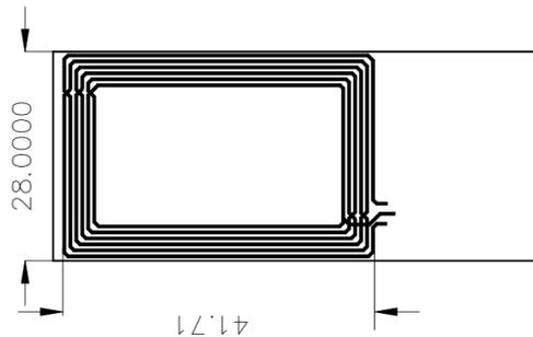
Antenna transmission frequency: 13.56MHz
