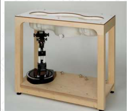
Figure 7.4.5-1: SAM Twin Phantom
