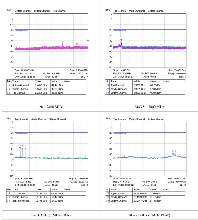
Figure 4: Emissions in non-restricted frequency bands
