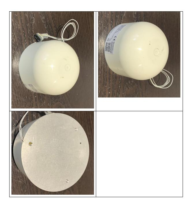
Note: serial cable connection is a test lead to allow radio to be put into continuous transmit mode for testing
