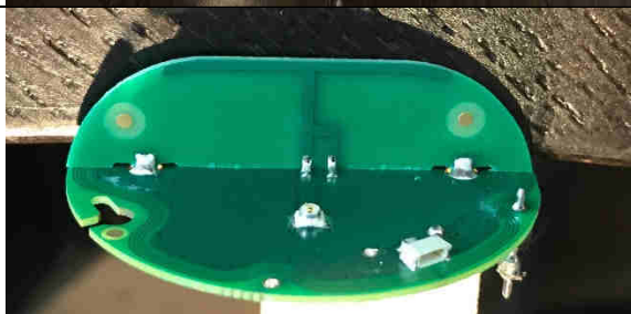
Antenna element PCB trace and feed point
