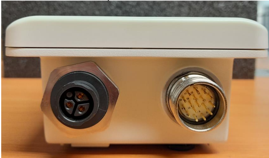
Figure 2.4: Three-pin Power input Connector (Black Connector to the left of the Multi-Pin Sensor Interface Port)
