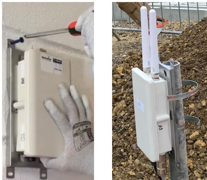
Figure 2.2: EdgeHub Bracket for Wall or Pole Mounting
