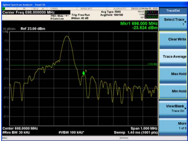
NB-IOT Band 71 QPSK 15kHz 1@11 CH-High
