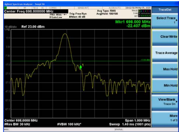
NB-IOT Band 71 BPSK 3.75kHz 1@47 CH-High
