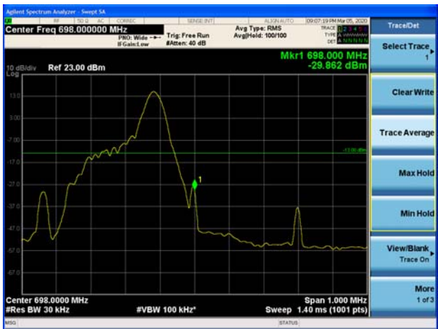
NB-IOT Band 71 QPSK 15kHz 12@0 CH-High
