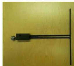
Figure 1 – MVG COMOSAR Validation Dipole
