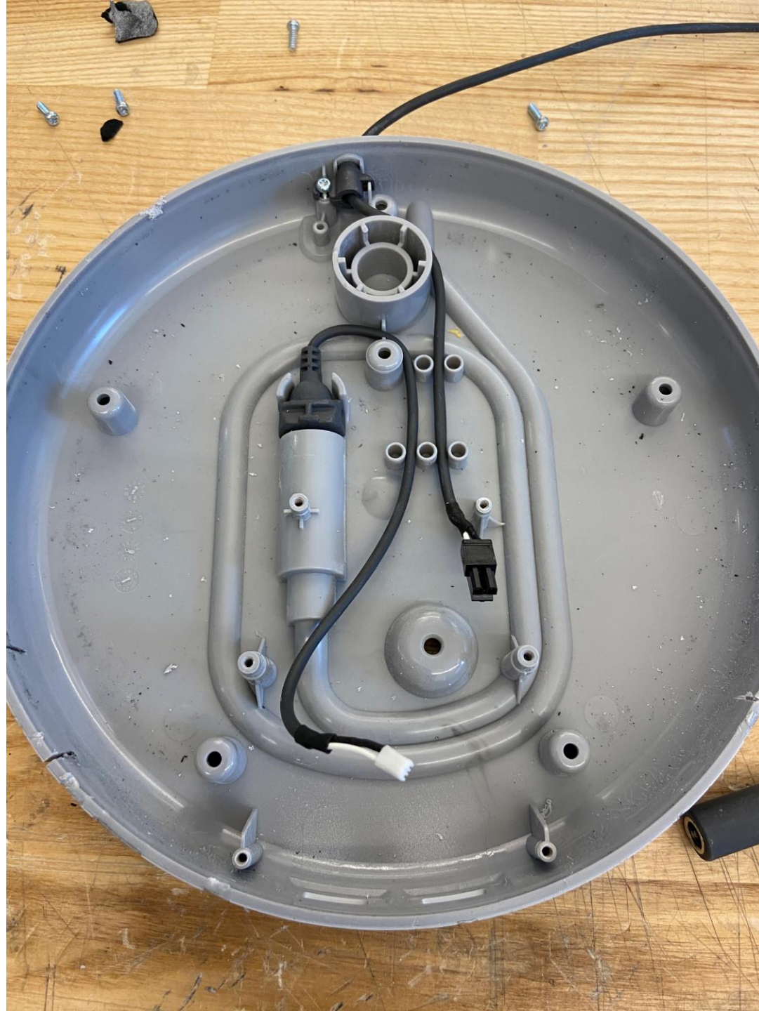
Fig 3. Inside of clamshell housing. Internal wire routing visible. Cable with black connector, connects to power supply, white connector plugs into PCBA, not shown here.
