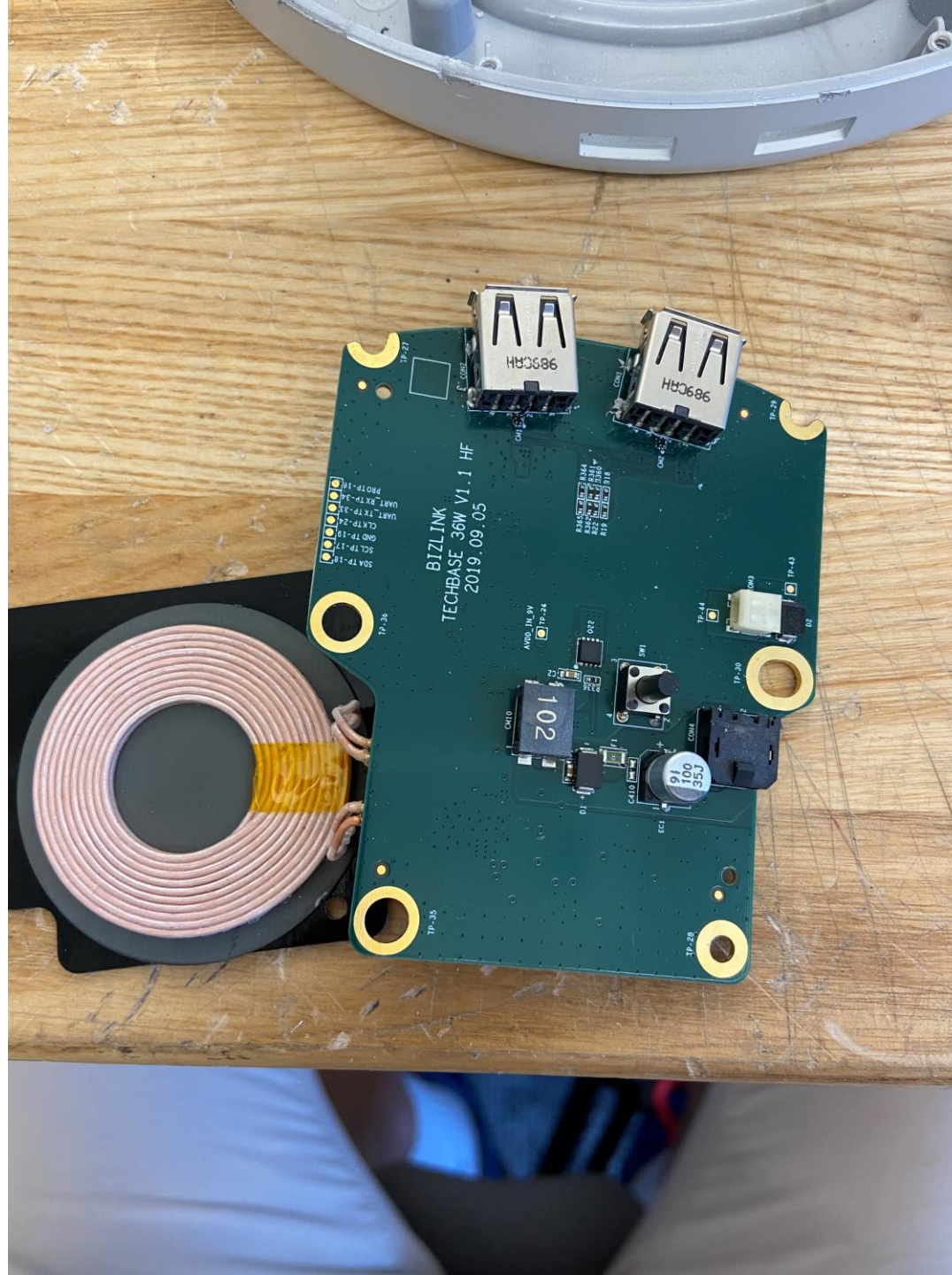
Fig 4. Bottom of PCBA w/ wireless charging module connected.
