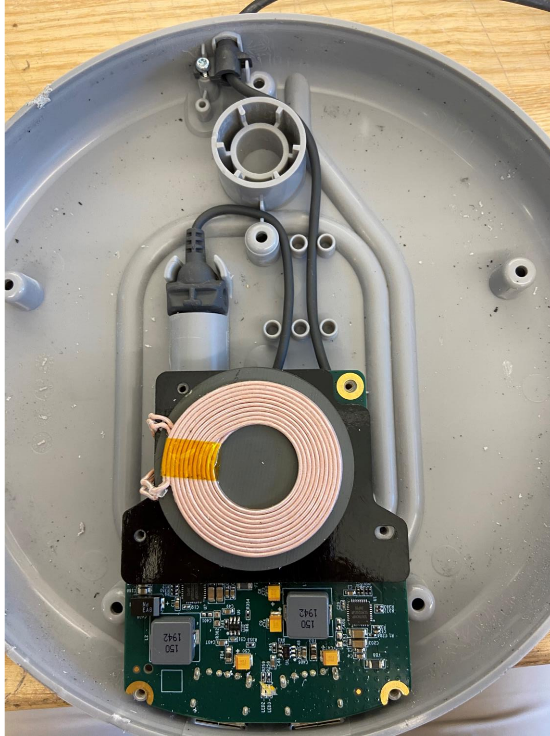
Fig 1. Inside of the Wireless Charging Desktop Base. Counterweight removed to reveal wire routing detail.
