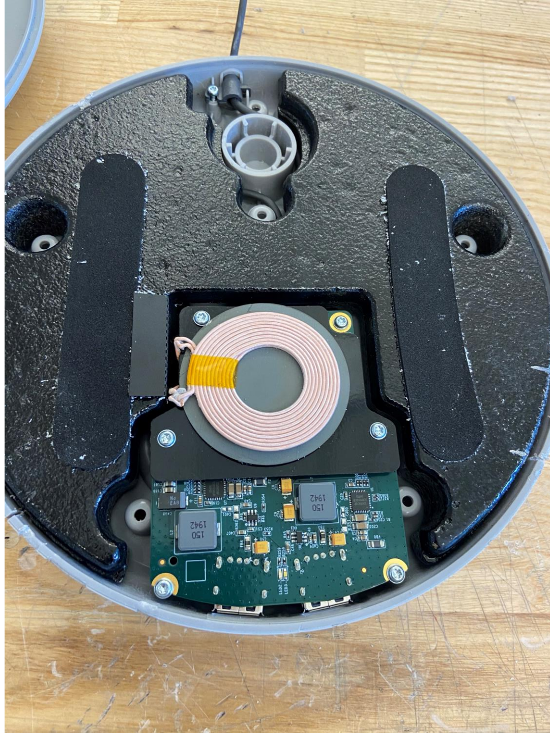
Fig 1. Inside of the Wireless Charging Desktop Base. Top clamshell housing removed. In view: cast iron counterweight, wireless charging module, PCBA.
