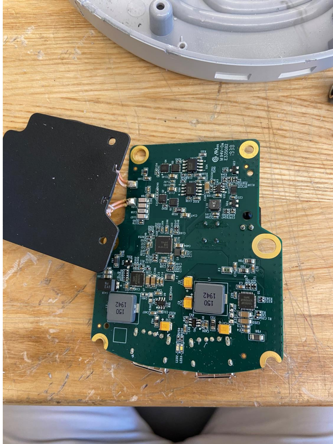
Fig 4. Top of PCBA w/ wireless charging module connected. Wireless charging module is affixed to a plastic support board.
