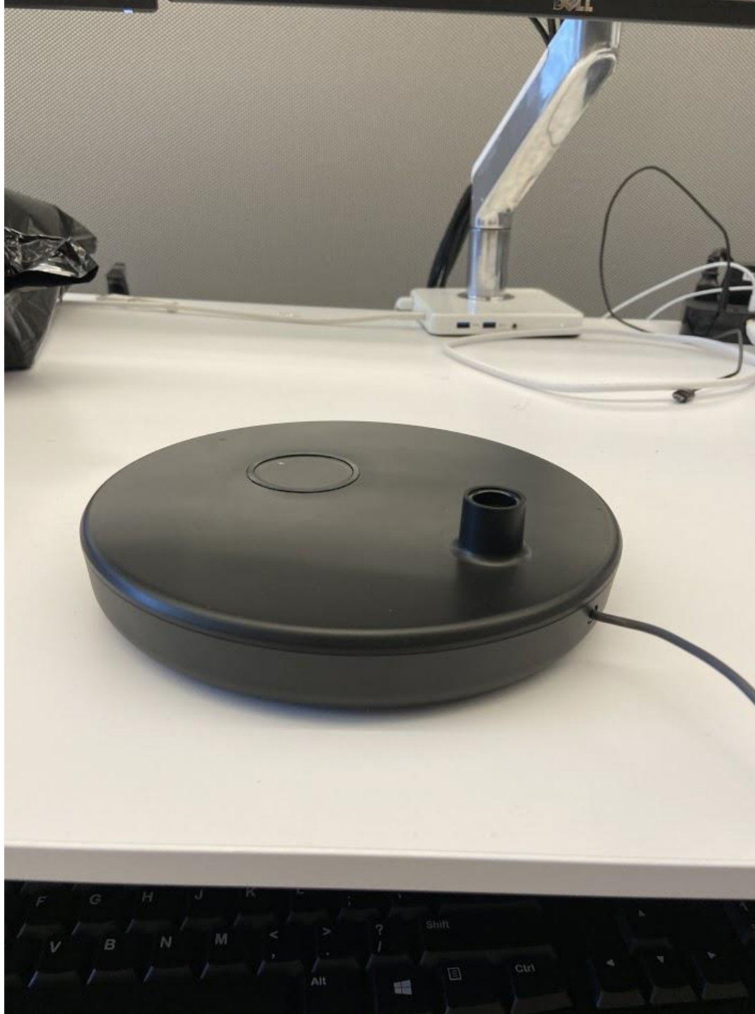
Fig 2. Back View, Wireless Charging Desktop Base for Nova Series Model N. Not Pictured: Nova Series Model N. External power cable Can be seen exiting base. Light body fits into stem.
