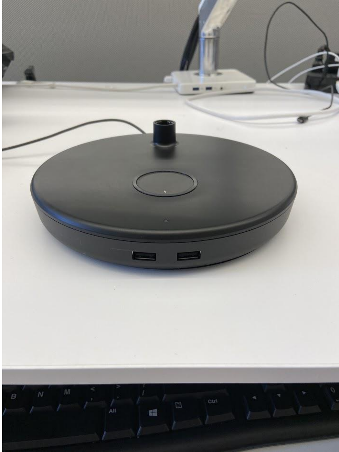
Fig 3. Front View, Wireless Charging Desktop Base for Nova Series Model N. Not Pictured: Nova Series Model N. USB Ports and wireless charging pad visible.
