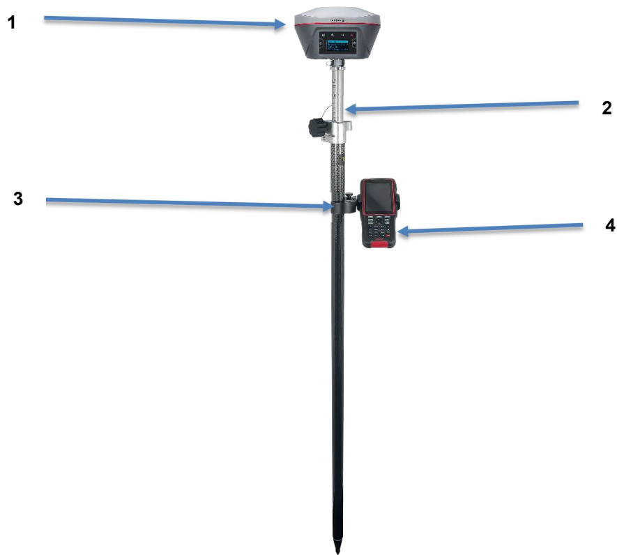
Figure 2.5 Oscar as a rover without radio antenna
