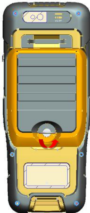
Figure 2.14 Remove the back cover
