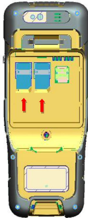
Figure 2.16 Put the SIM card in the holder
