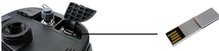
Figure 2.13 Connect Oscar to a USB memory stick
