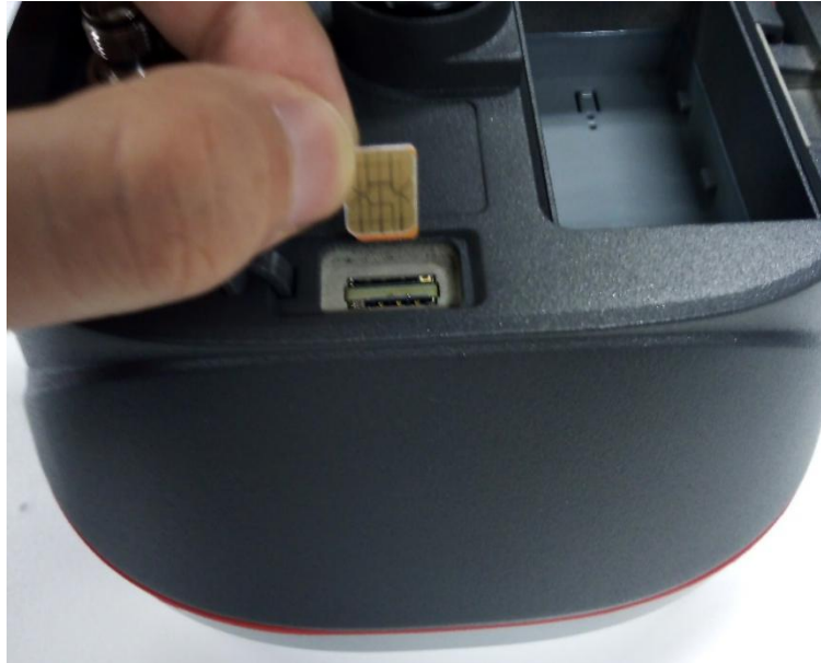
Figure 2.3 Insert the SIM card
