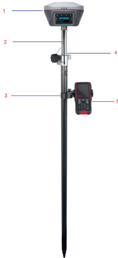
Figure 4.10 Oscar as a Rover – Internal Radio
