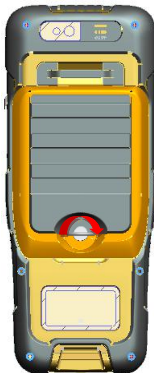
Figure 2.18 Insert the back cover
