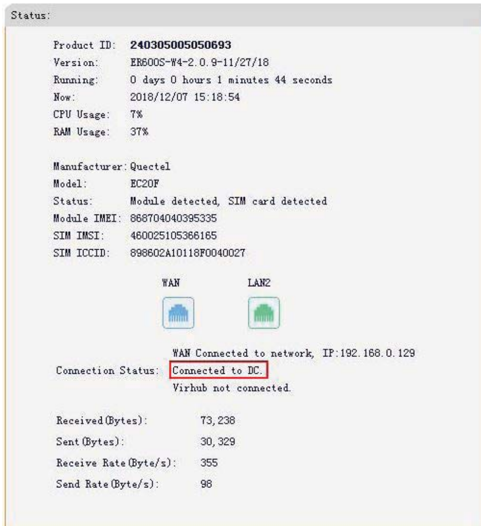
Figure Appendix 4-4: DTU connected to DC
