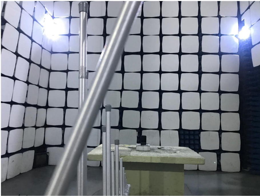
Radiation Emission Test Setup (30MHz to 1GHz)
