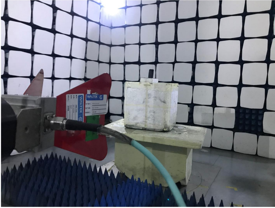
Radiation Emission Test Setup (1GHz to 18GHz)
