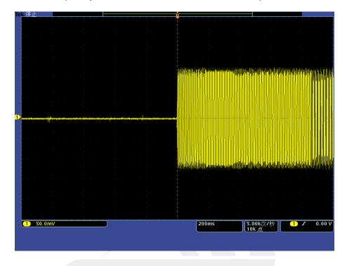
Transmitter Frequency Behaviour @ 25.0 KHz Channel Separation-----On - Off
