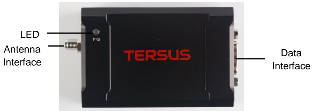
Figure 23 RS900C 1W Radio Station
