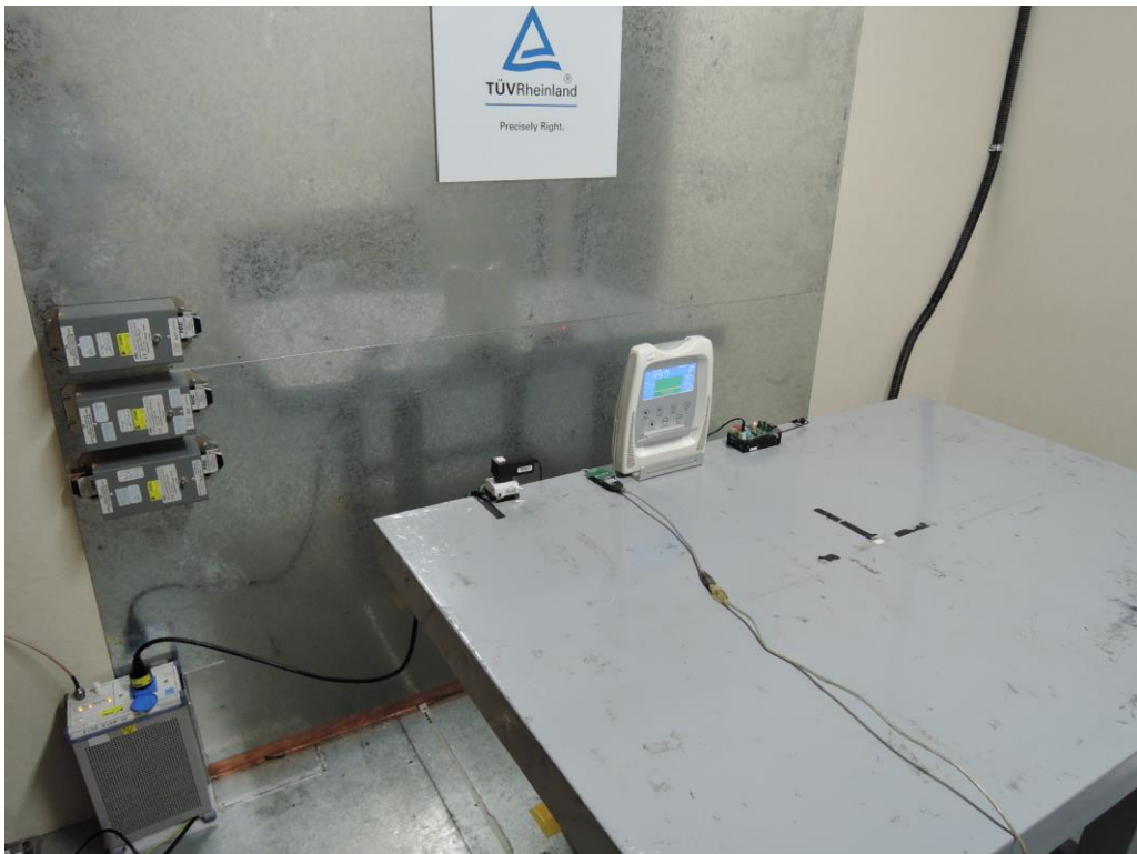
Photograph 7: Set-up for for Mains Conducted testing Front
