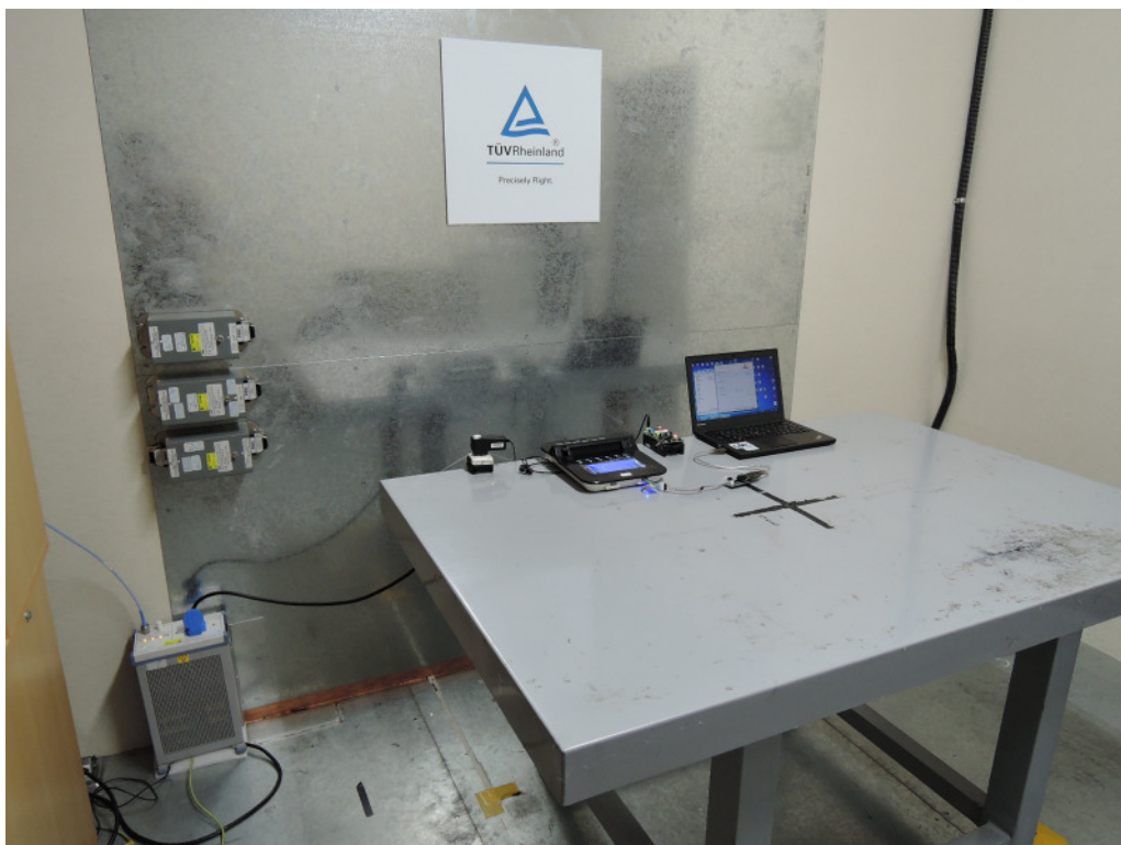
Photograph 7: Set-up for for Mains Conducted testing Front
