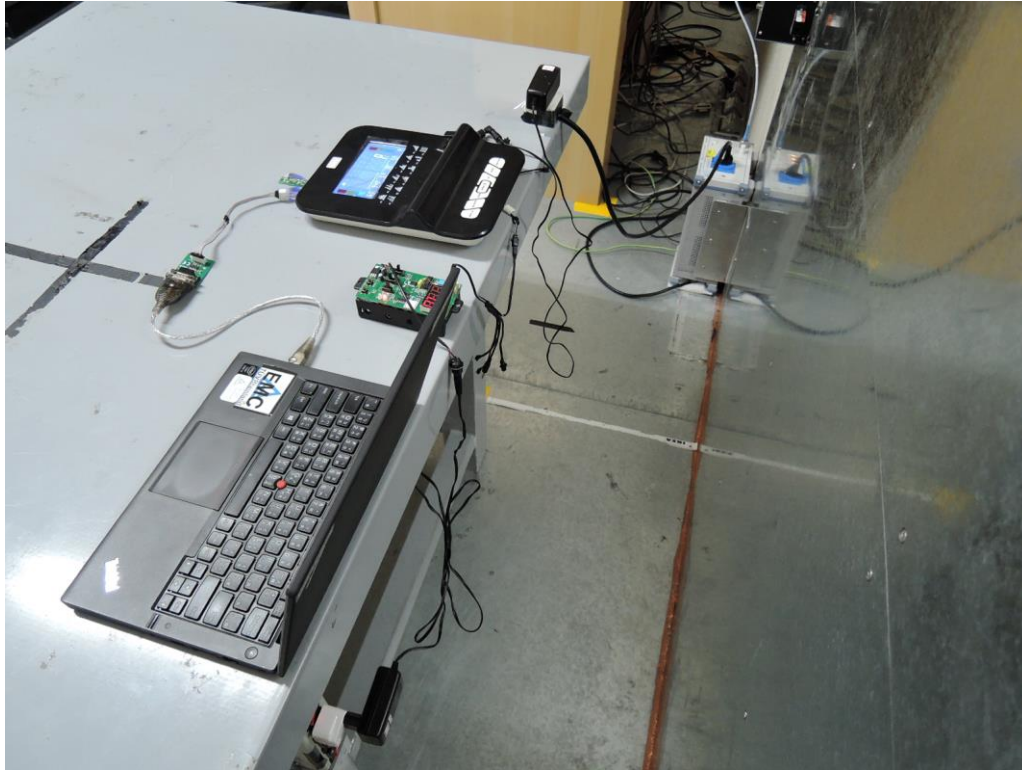
Photograph 6: Set-up for for Mains Conducted testing Back
