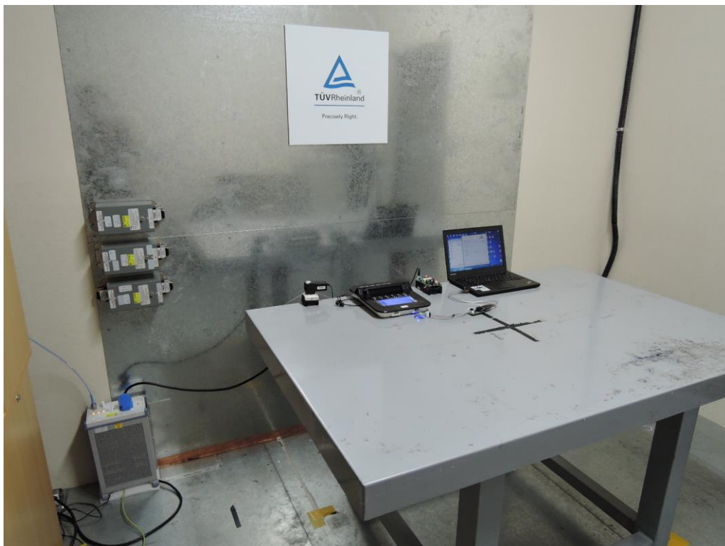
Photograph 7: Set-up for for Mains Conducted testing Front
