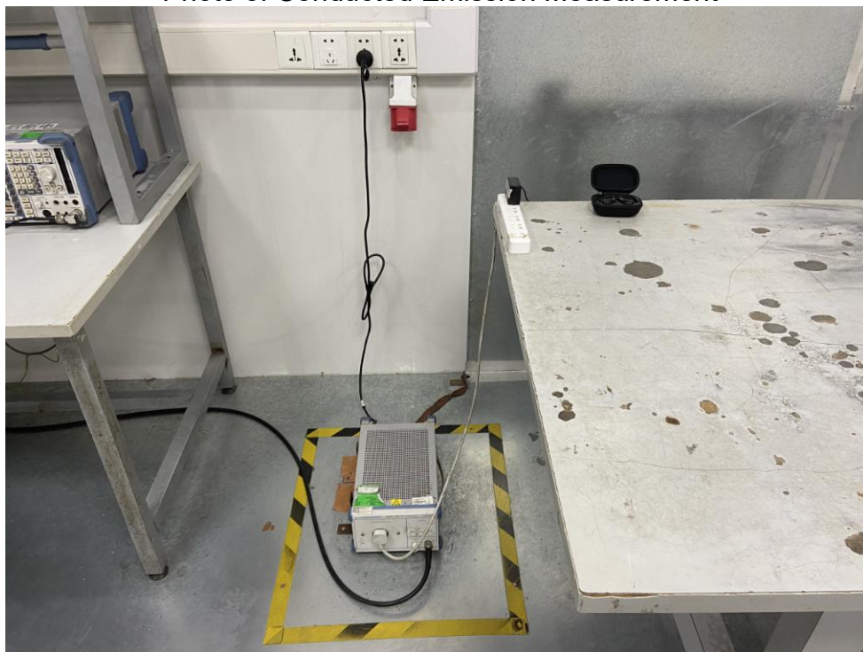
FCC ID: 2AMD8Z12409 Photo of Conducted Emission Measurement
