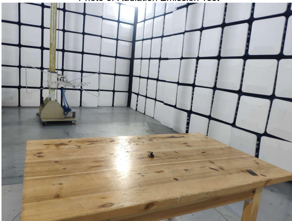
Photo of Radiation Emission Test
