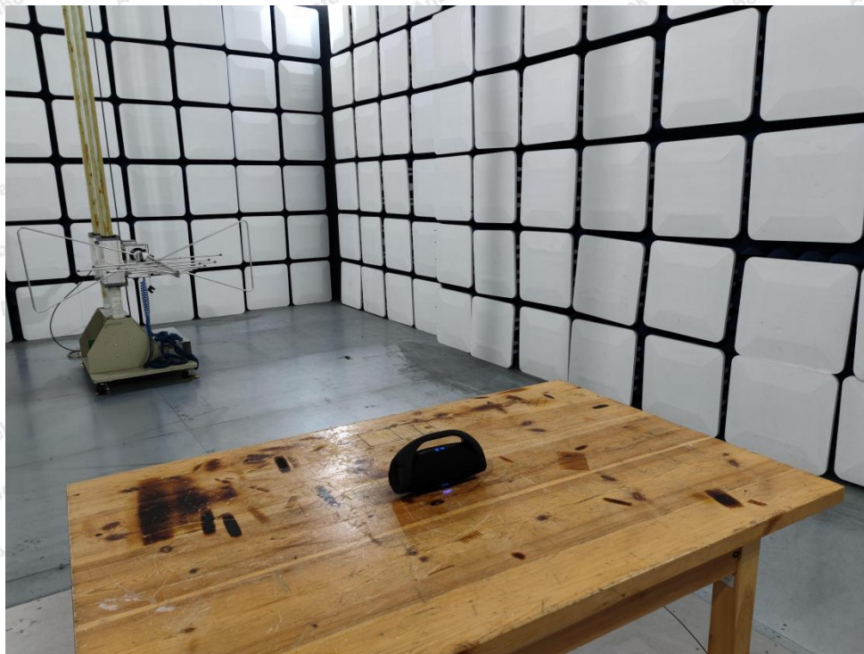
Photo of Radiation Emission Test
