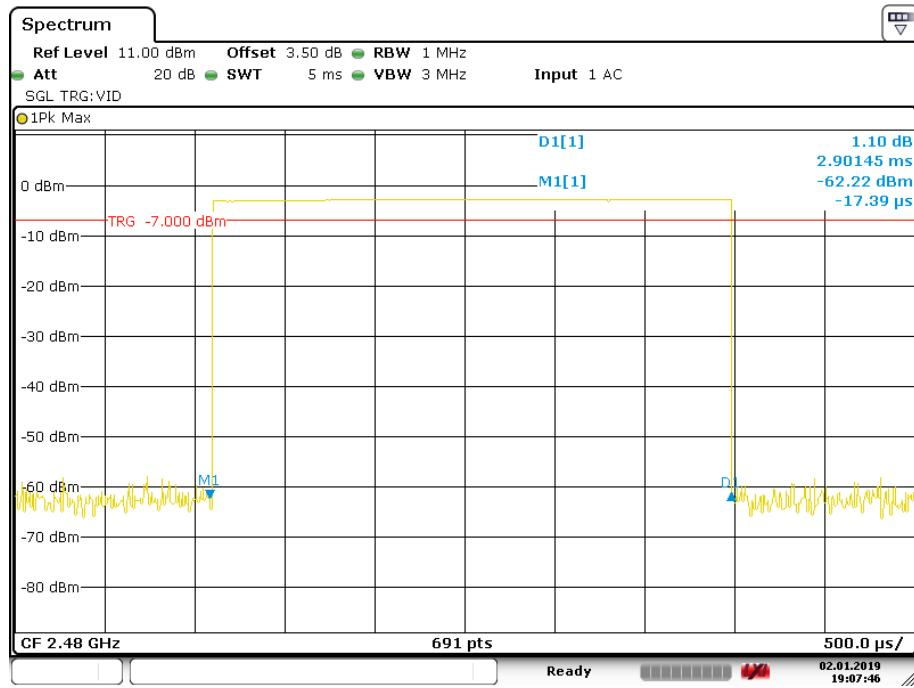
**EDR ( $\pi/4$ -DQPSK):****Pulse time, Low Channel, 2DH1**
