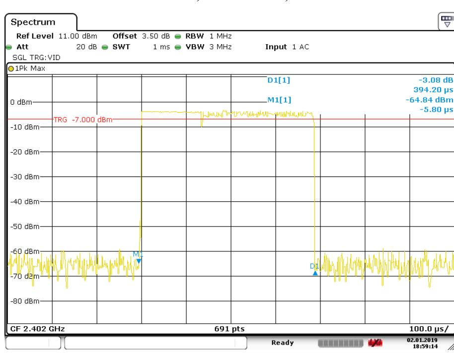
**Pulse time, Middle Channel, 2DH1**
