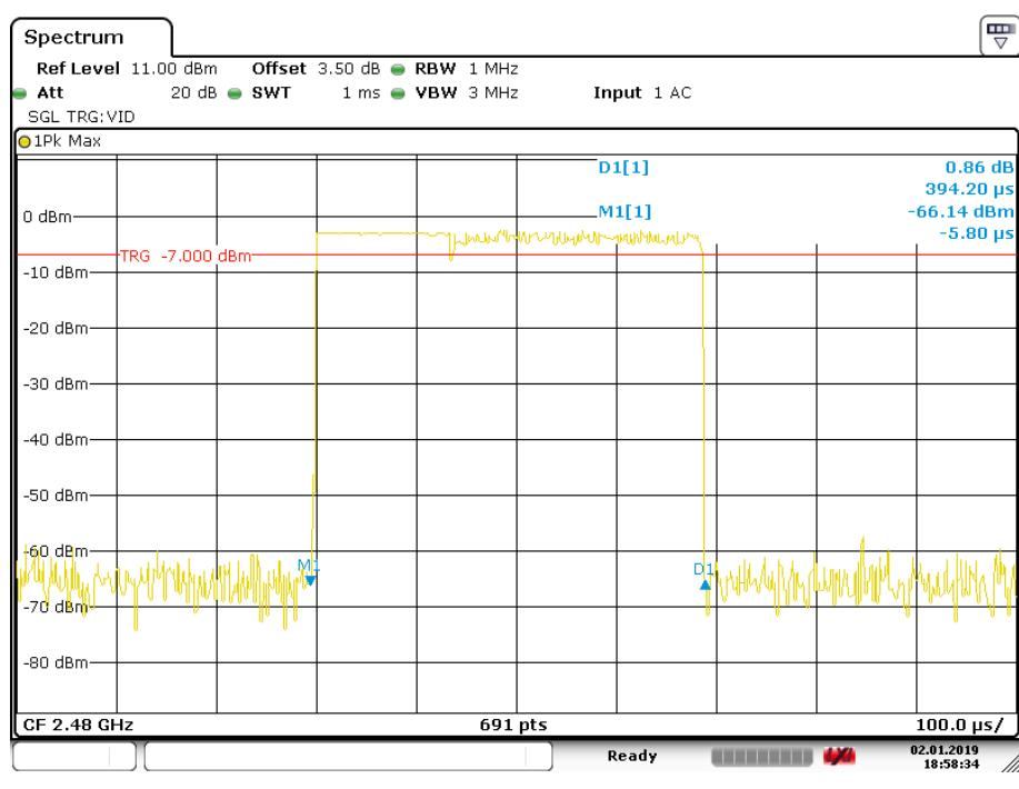
**Pulse time, Low Channel, 2DH3**
