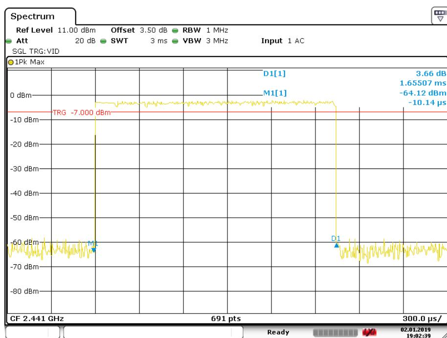
**Pulse time, High Channel, 2DH3**
