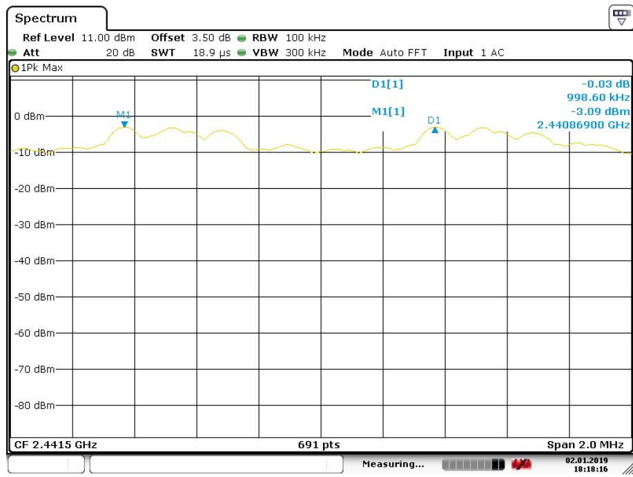
**EDR ( $\pi/4$ -DQPSK): High Channel**
