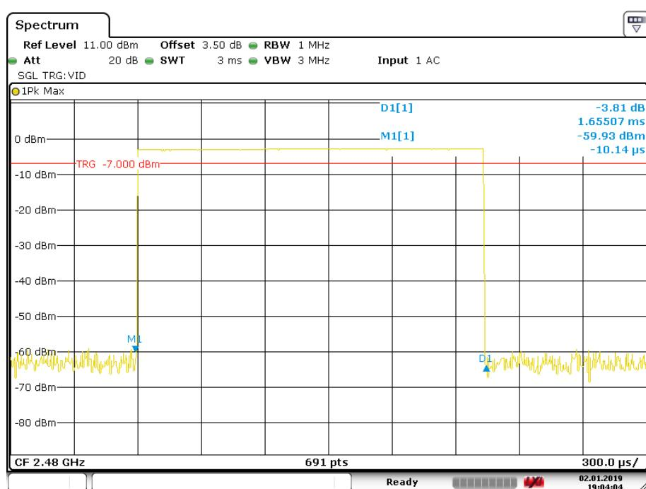
**Pulse time, Low Channel, DH5**
