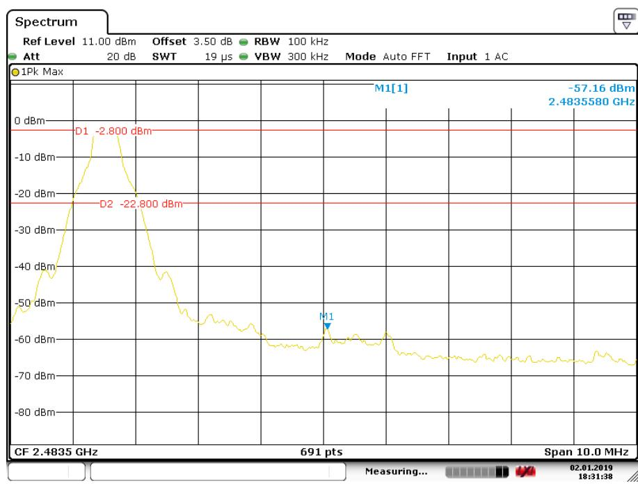
**EDR ( $\pi/4$ -DQPSK): Band Edge-Left Side Hopping**
