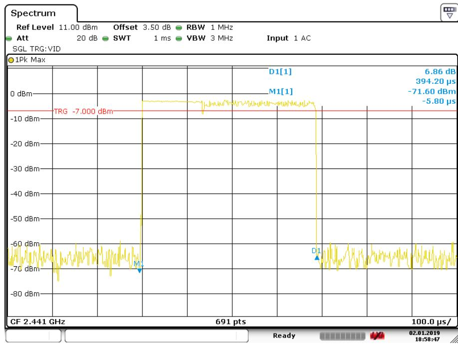
**Pulse time, High Channel, 2DH1**
