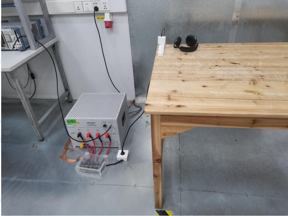
Photo of Conducted Emission Measurement
