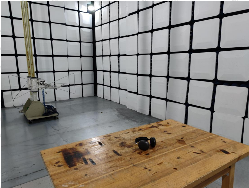
Photo of Radiation Emission Test
