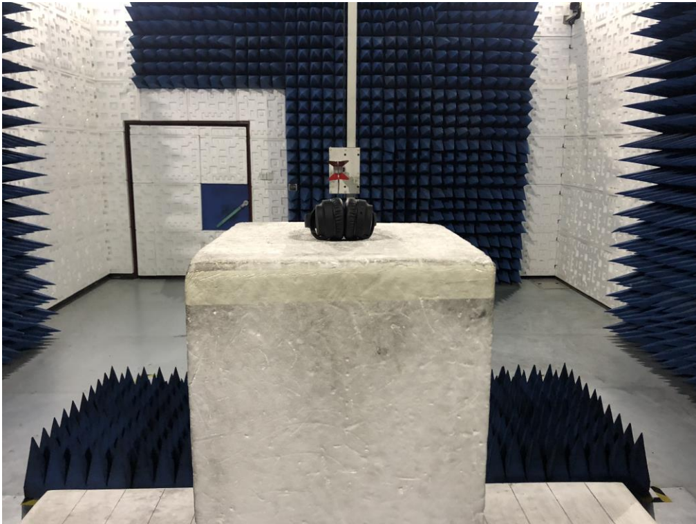
RADIATED EMISSION TEST SETUP ABOVE 1GHZ
