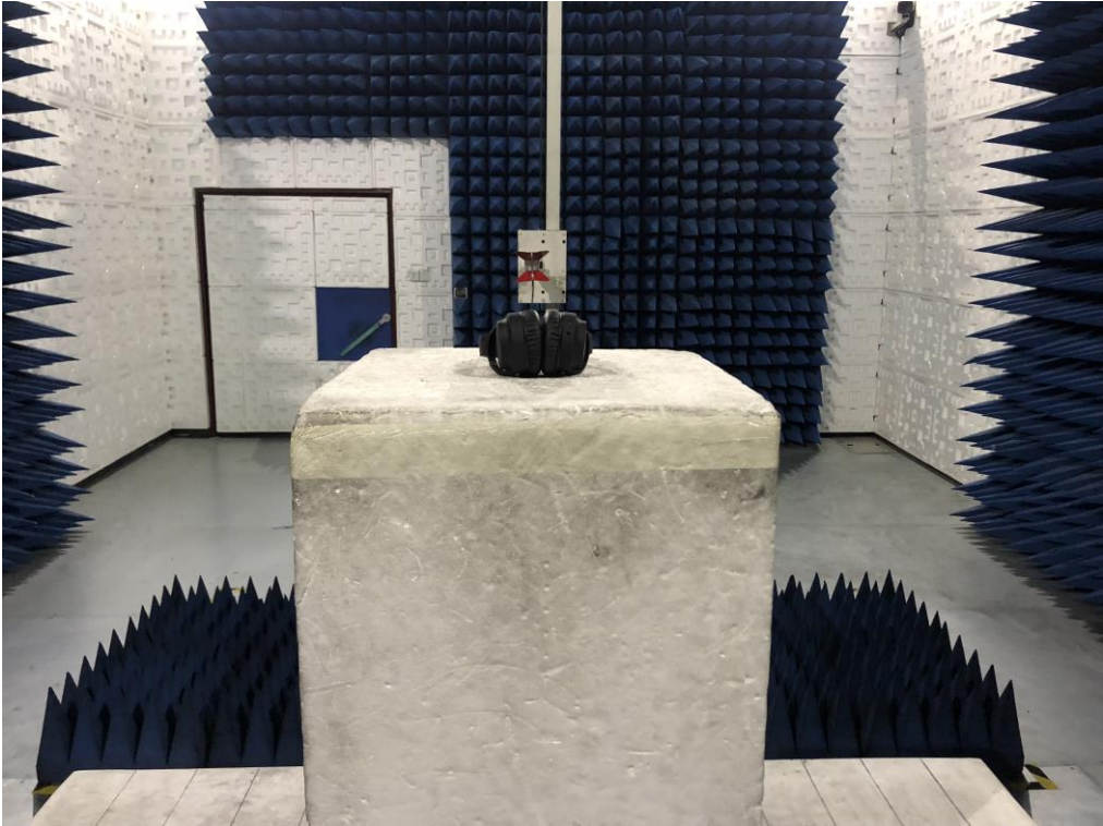
RADIATED EMISSION TEST SETUP ABOVE 1GHZ
