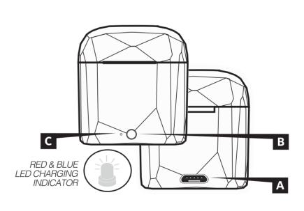
A MICRO-USB CHARGING PORT B POWER BUTTON LED INDICATOR
