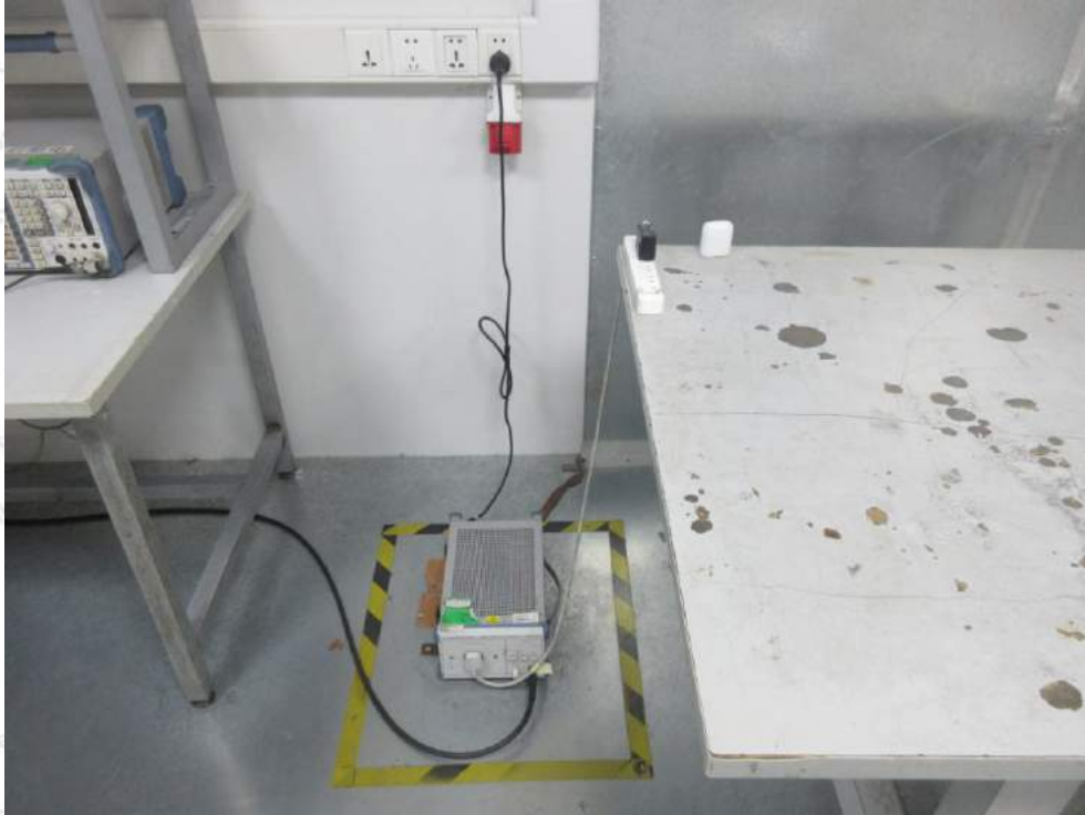
Photo of Conducted Emission Measurement
