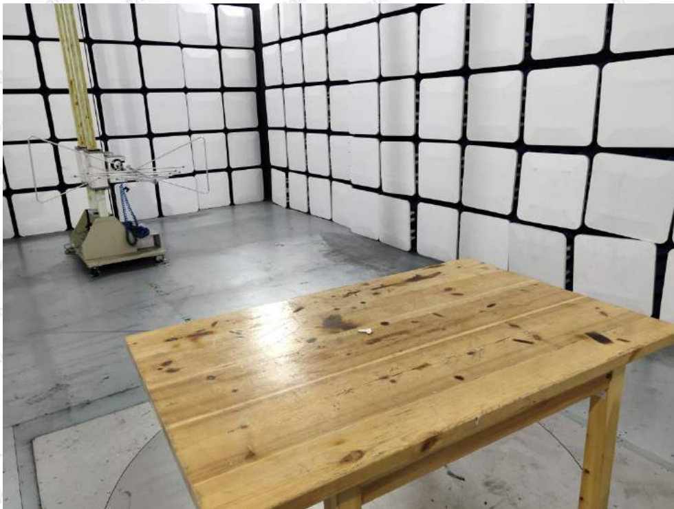
Photo of Radiation Emission Test
