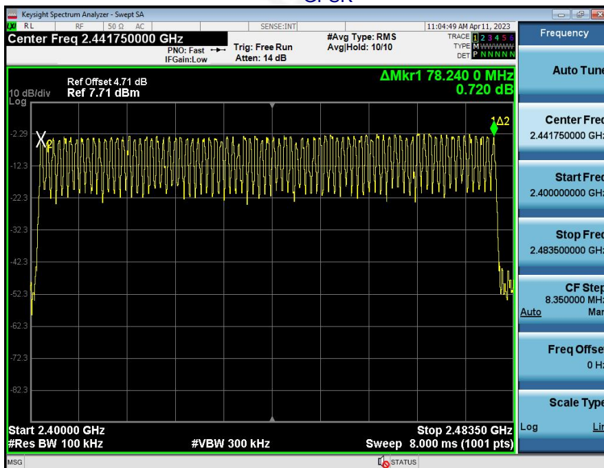
Test Plots: 79 Channels in total GFSK
