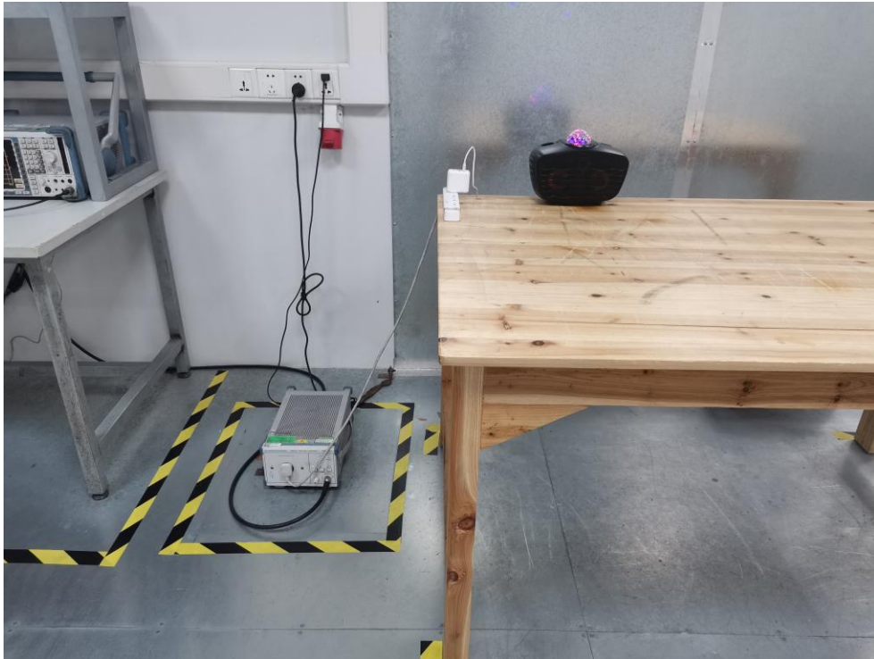
Photo of Conducted Emission Measurement
