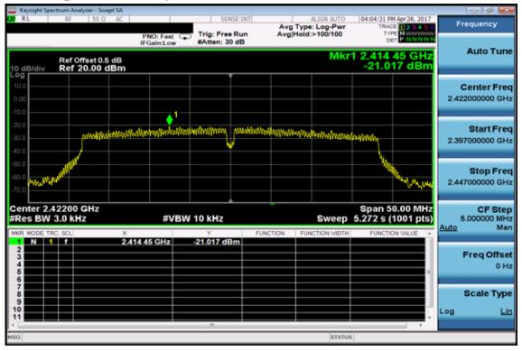
**Power Spectral Density Test Plot (CH-Mid)**
