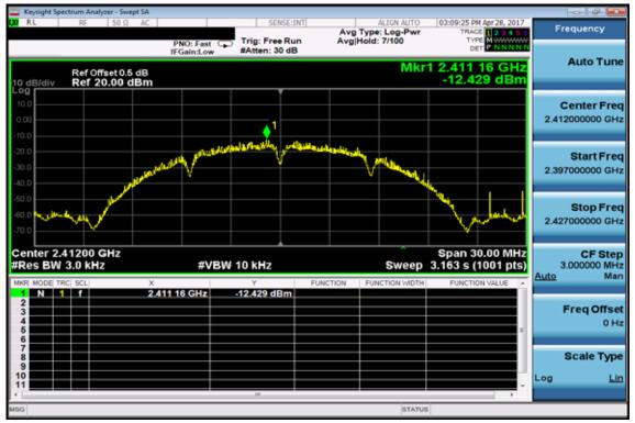
**Power Spectral Density Test Plot (CH-Mid)**
