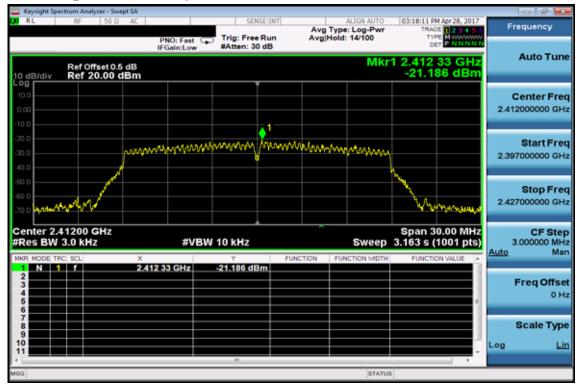
**Power Spectral Density Test Plot (CH-Mid)**
