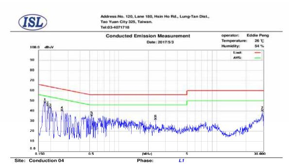
Limit: CISPR22 Class B Conduction(QP)
