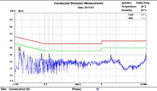
Limit: CISPR22 Class B Conduction(QP)
