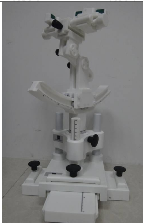
COMOSAR Mobile phone positioning system
