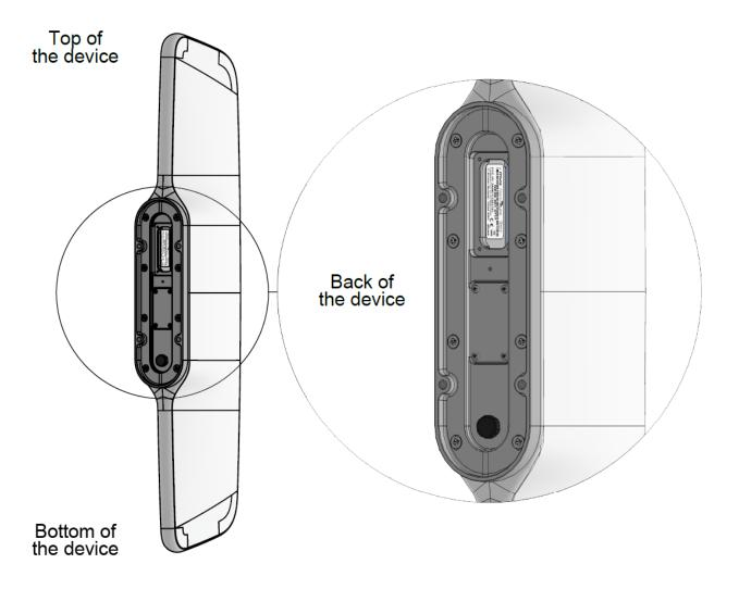
The FCC ID label is located in the connectors (power supply, Ethernet) compartment. The plate (cover of the connectors compartment) in which the cable (or the cables) pass through, is not assembled to the device when it is shipped from the factory. The user has to plug at least one cable (PoE) to operate the device. At this time, the FCC ID indicated on the label, which is glued on one side of the connectors compartment, is visible to the user.
